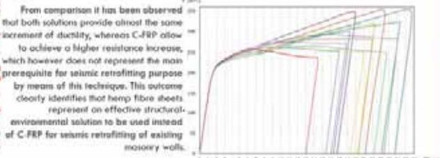
The obtained results have shown that, referred to the seismic performance of the unreinforced wall, a maximum strength increase of 2.42% and 11.18% and a maximum ductility increase of 35.84% and 39.33% have been obtained with H-FRP and C-FRP, respectively.
