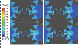
results obtained are a time dependent comparison of the flow rate trend in function of the gap variation. Is possible to observe that the accuracy of the simulation increases with the leakage reduction and the computational cost
