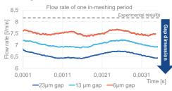
The numerical leakage is the key parameter for the CFD analysis of a gear pump and by estimating the discretization error is possible to redesign the pump without the construction of prototypes.
