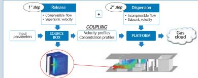
In a nutshell: The accidental phenomenon (highly pressurised gas release) is split in two phases  $\rightarrow$  supersonic release and dispersion.
